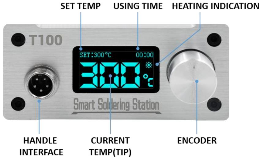
Fig 5.1 front panel
